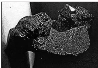
Fig. 11. Pommel section removed for metallurgical examination.
